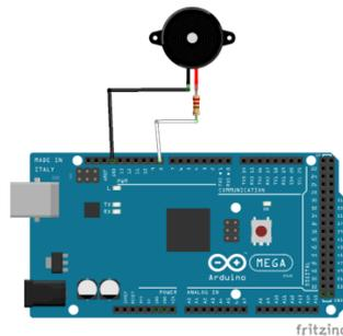
Gambar 13. Rangkaian Buzzer
