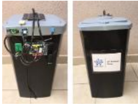
Figure 12: Smart Bin Management System
