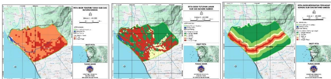
Figure 4. Spatial Distribution of (a) Soil Texture, (b) Land Cover, and (c) Distance from the River Network
