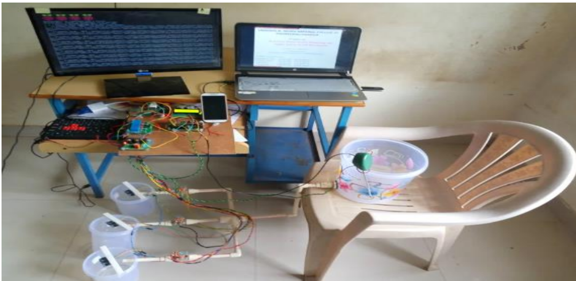
Figure 10 Complete Setup Of IoT water level Monitoring System
