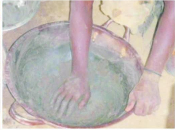
Fig.5: Panning of gold to reduce impurities
