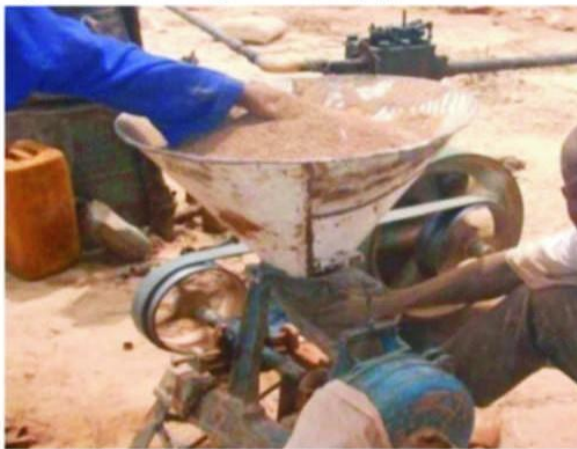
Fig.4: Locally fabricated grinding mill
