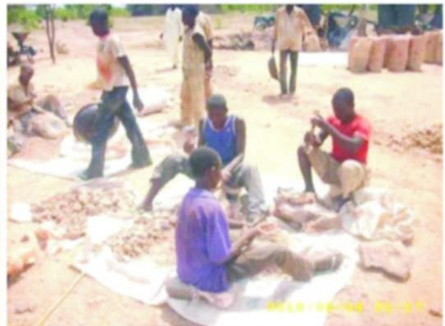
Fig. 3: Breaking of gold mineral ore into pieces
