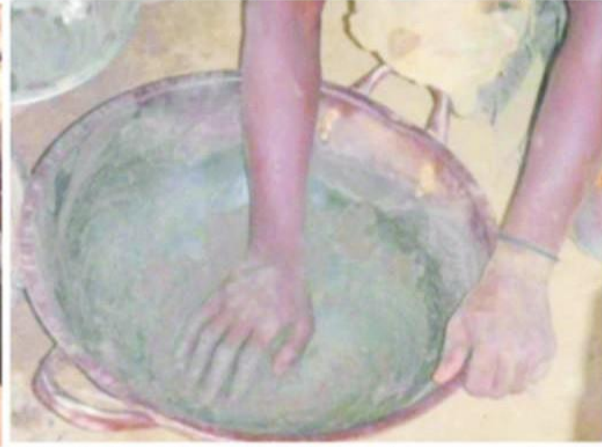
Fig.5: Panning of gold to reduce impurities
