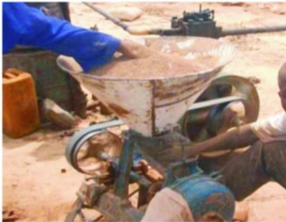
Fig.4: Locally fabricated grinding mill
