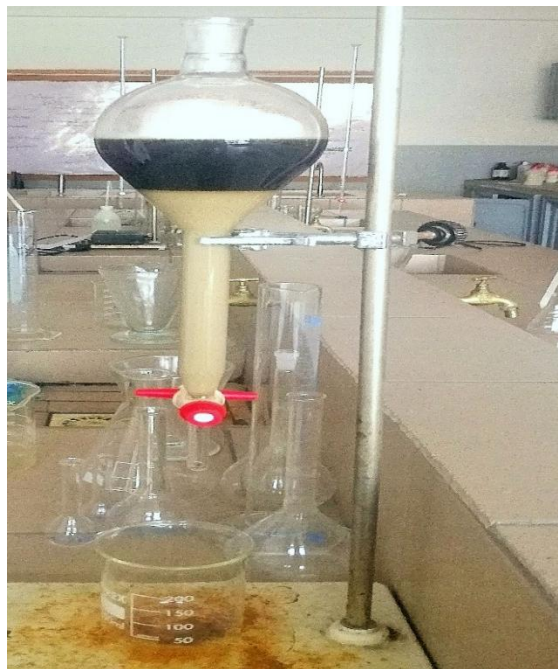
Fig. 11: Decantation of the pyrolytic oil.
