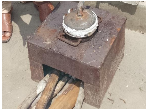
Fig. 7: Tank sealed with silicone
