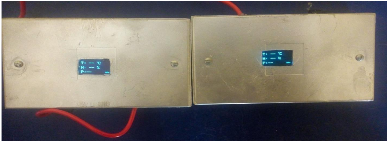
Figure 17. Showing When both the server and Receiver is On, but the reading are not displaying on the screen because they are not with the coverage area of the server
