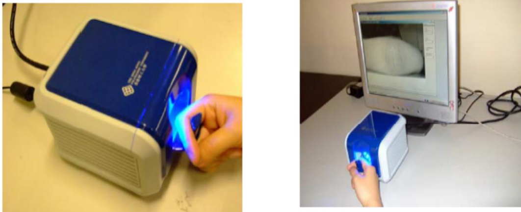
(a) The outlook of the developed FKP image acquisition device (b) The device is being used to collect FKP samples
