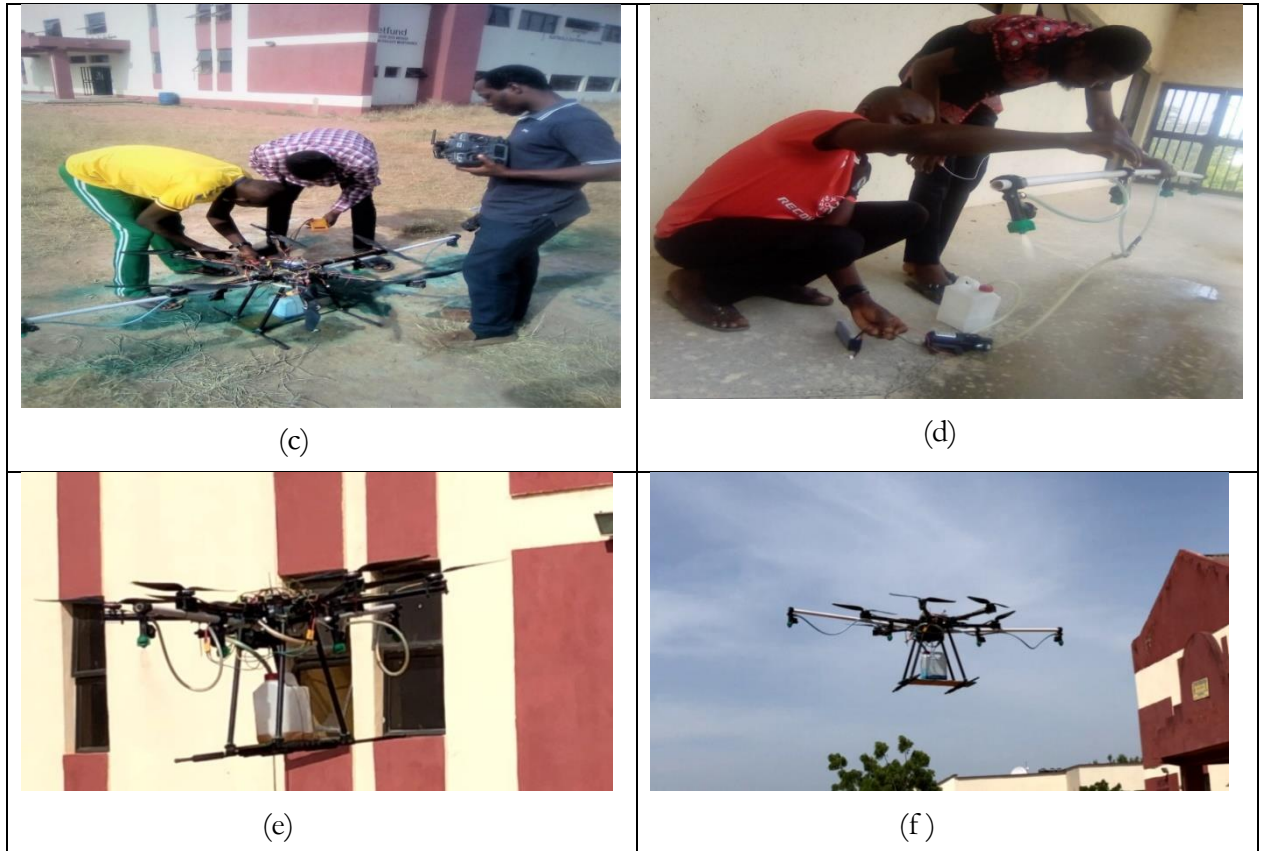
Figure 1.5: (a) Heritage Agricultural Spraying Drone ready for testing (b) Shows the Pixhawk flight controller displaying blue light it is powered properly connected for usage (c) Shows the battery level of the sprayer pump being tested (d) Shows the locally assembled agrochemical sprayer being tested before mounting on the drone, (e) & (f) shows the UAV sprayer in action.
