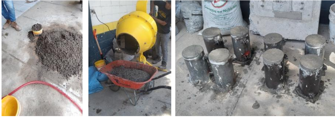
Figure 1. Process of making concrete with PET.
