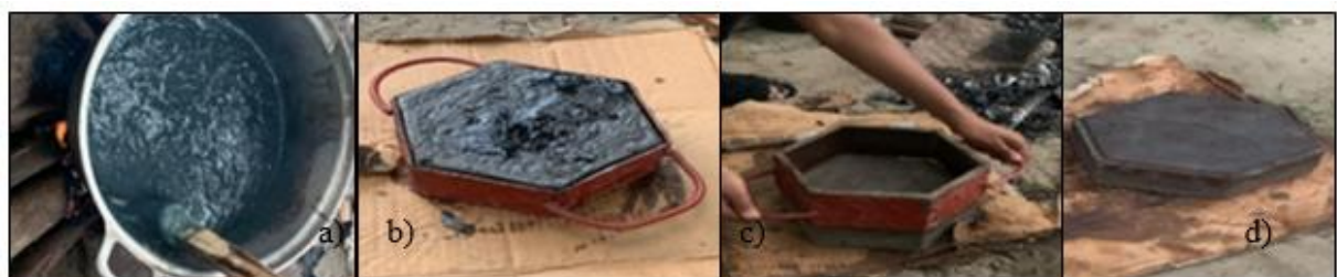
Fig. 2: a) Molten plastic b) Molded paving stone c) Demolding d) Finished paving stone
