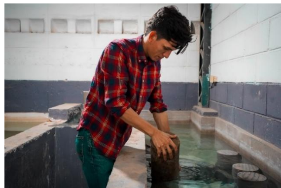
Figure 2. The cylinders were removed from the water to conduct strength tests, which were performed at 7 and 28 days of curing.
