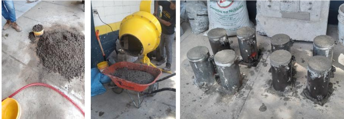
Figure 1. Process of making concrete with PET.
