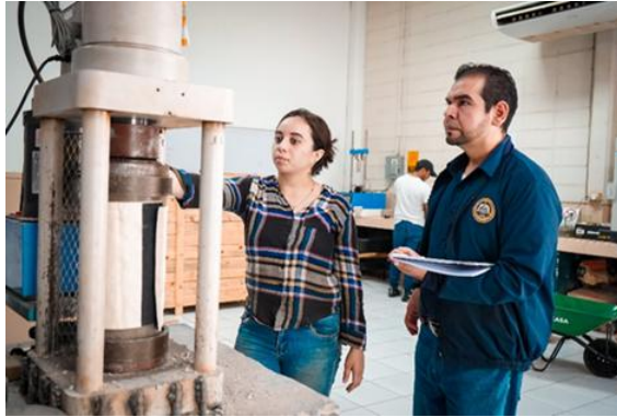
Figure 4. Data collection from concrete cylinders subjected to compression testing.
