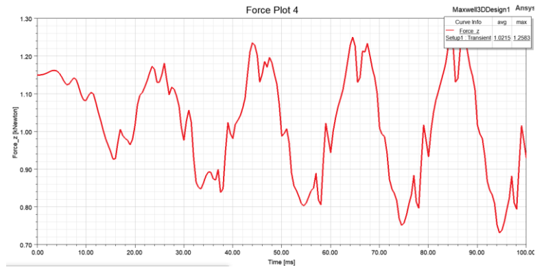
Figure 19: Radial forces at LV on short circuit condition
