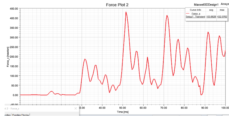
Figure 17: Radial forces at LV on normal condition
