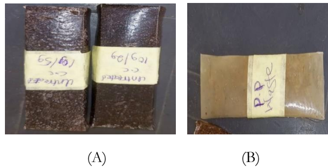
Plate 1: (A) Treated Cocoa fruit shell and unused polypropylene composites, (CFS) (B) Only polypropylene waste
